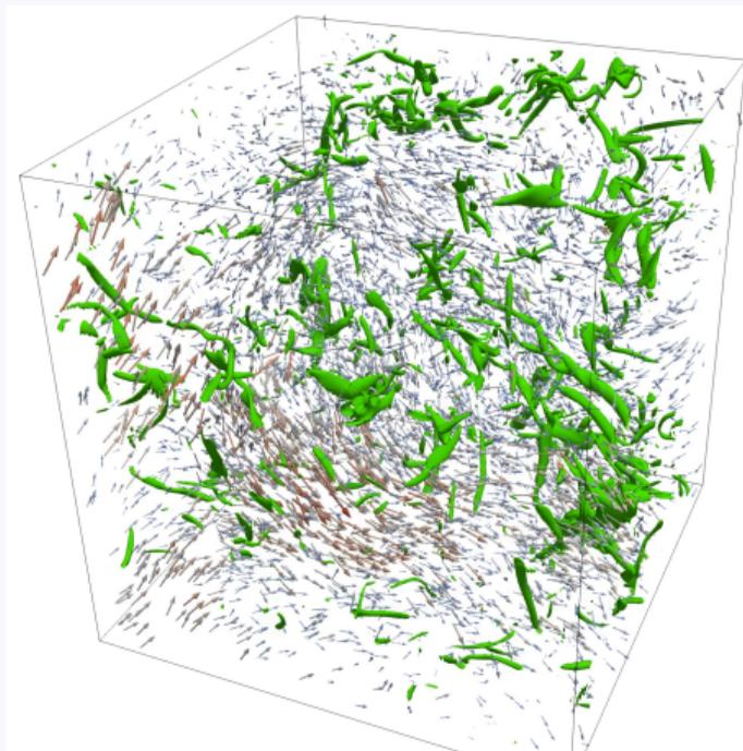
Velocity field and iso-surface of  $|\boldsymbol{\omega}|^2$
