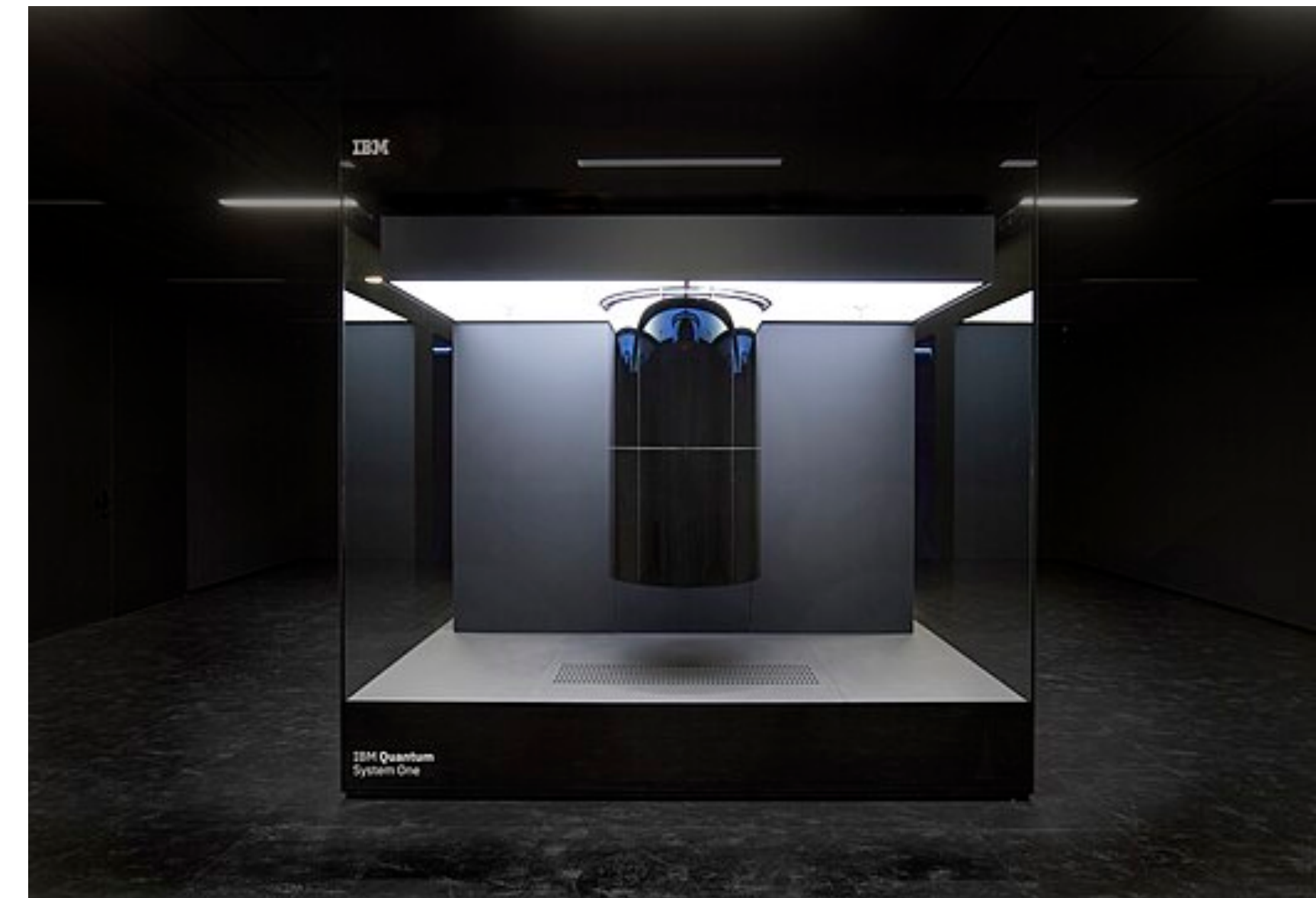
IBM, 20 superconducting qubits [figure from wikipedia “Quantum computing”]
